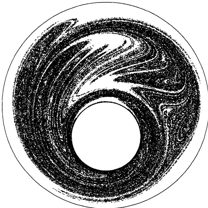
FIGURE 5. Viscoelastic simulation in the Stokes limit for  $\theta = \frac{3}{2}\pi$  and  $\Omega < 0$ ;  $We = 10^{-3}$  and  $Re = 10^{-3}$ .
